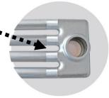
The internal grinding machine, specifically developed for the tube radiator production, will now make it possible to grind welded radiator elements at their **head-end tube weld seams** efficiently and in **top quality**, i.e. in the internal area that is particularly difficult to access.
