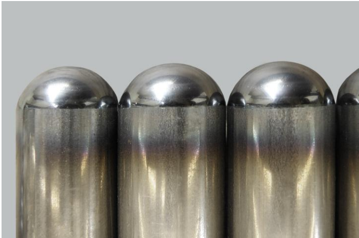
Image2: Since the workpiece does not move, it also possible to process geometries that are not rotationally symmetrical
